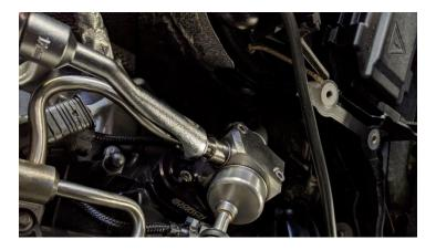
**NOTE:** We don't expect everyone to have specialty sockets for proper torque spec. In this case, simply "snug" the nuts with a 17mm wrench. 31nm is NOT a lot of torque to be sure to not over tighten and damage the line.
