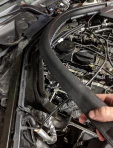
3. Remove the ECU cover by first unclipping the coolant line and then pulling directly up on the cover:
