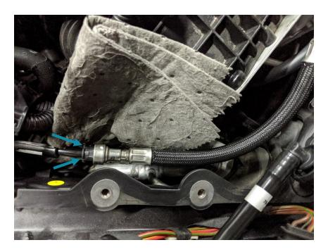
14. Lastly, remove the OEM high pressure pump using a T30 socket. Use **CAUTION** when removing the pump. The area must be VERY clean to avoid contaminating the pump and engine. You also must unthread each mounting bolt a little at a time to ensure the pump comes out STRAIGHT.
