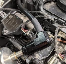
Once the collars are fully threaded on, use a wrench to tighten them. You may need to hold the hose in place by using an additional wrench on the hex portion of the hose fitting.
