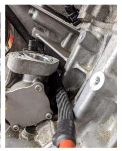
Once routed properly, clip the line into the OEM fuel line (where the hardline was removed from in step 15).
