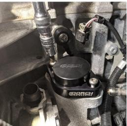
19. Now remove the alignment tool and insert the Dorch Engineering fuel pump. Use extreme **CAUTION** when installing the pump. The bolts MUST BE TIGHTENED EVENLY. Uneven loading of the spring can damage the pump. Also, be **EXTREMELY CLEAN** as all HPFPs are very sensitive to contaminants.
