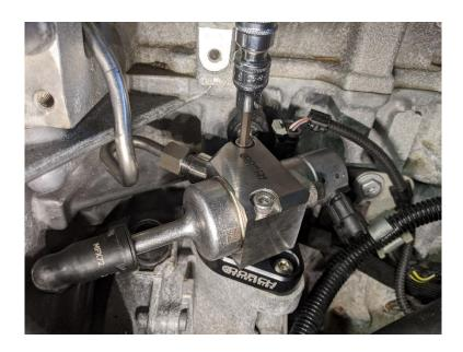
Lightly apply oil to the threads of the HPFP to prevent galling. If the nuts thread on effortlessly and bottom out with all the fittings well aligned, the nuts can now be torqued (a 17mm wrench can be used for this if need be, since special sockets are required for proper torque). Be sure not to over tighten the nuts.
