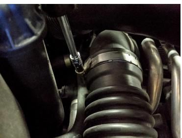
8. Next remove the four 10mm bolts holding on the throttle body along with the electrical connector and vacuum line:
