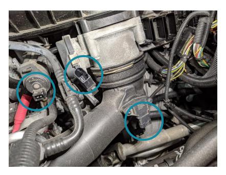
6. Remove the 2 vacuum connections pictured below and then unclip the line and purge valve from the intake manifold:
