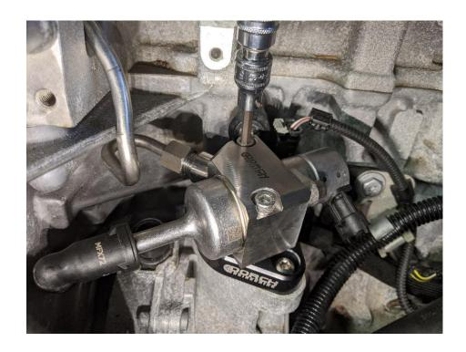
Lightly apply oil to the threads of the HPFP to prevent galling. If the nuts thread on effortlessly and bottom out with all the fittings well aligned, the nuts can now be torqued (a 17mm wrench can be used for this if need be, since special sockets are required for proper torque). Be sure not to over tighten the nuts.
