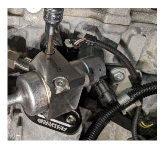
21. The low pressure hose can now be routed into it's final position and clipped into the OEM hose. The Dorch low pressure hose simply slides right into the OEM BMW hose. It may take some effort, but it will click in. Once it clicks in, it will not pull out. The gray clip can then be re-installed on the OEM BMW hose (Ref. Step 15).
