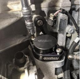
19. **BEFORE** inserting the HPFP into the flange, push the low pressure hose on to the Dorch HPFP inlet. You will need to unthread and remove the locking collar, slide the hose onto the pump, and then re-install the locking collar. The HPFP can then be dropped into place in the flange.
