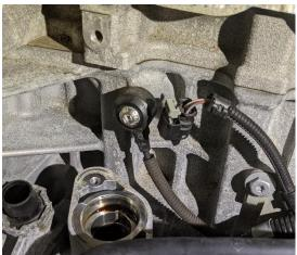
14. Now remove the OEM low pressure hardline hold-down clamps. Remove the two 13mm bolts below the cable junction assembly:
