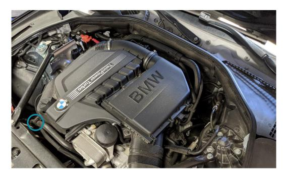
2. Next the airbox needs to be removed. First loosen the 7mm hose clamp and unplug the MAF, then lift the 3 main harness clips off the back corner of the airbox. Now lift up firmly and away from the fresh air inlet.
