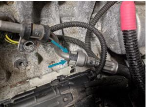
15. The low pressure line can now be removed. Be sure to place a rag under the quick-connect fitting before removal. This fitting requires removal of the gray clip first, and then push the black plastic collar in, while simultaneously pulling the line off (pictured above)
