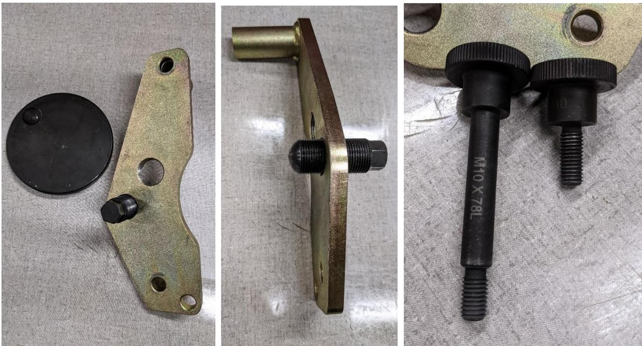
To fasten the tool to the engine, you will need the two thumb screw fasteners pictured above, right.
