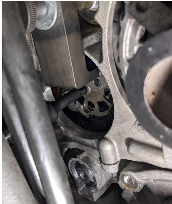
Once the tool is properly locked into the timing gear, use a T55 socket to crack loose the center bolt. Once it is cracked loose, do not remove the bolt. Instead, put it on finger tight and remove the locking tool.
