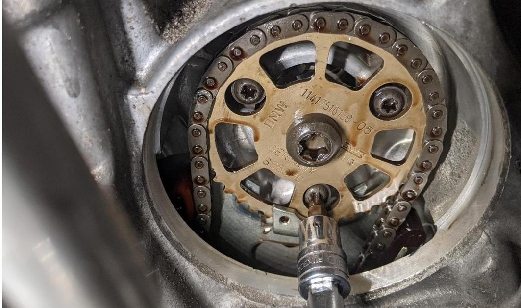
37. Now using a flat head screwdriver, very carefully depress the timing chain tensioner (pictured on the left below). Hold the screwdriver in place and then slide the timing gear off the tip of the Vacuum pump shaft. Once the gear is off the shaft, release the screwdriver and allow the gear to rest as pictured (right):
