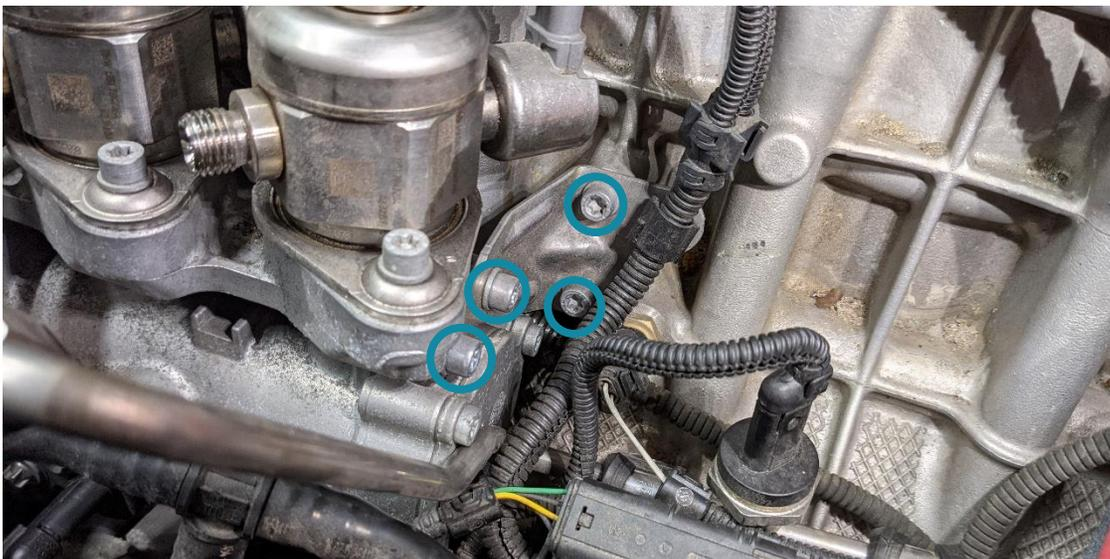
36. Once again, using a 22mm socket on the crank pulley, rotate the engine clockwise until the 3x T30 bolts behind the timing gear line up with the three circular holes. Once these are lined up, use a T30 socket to loosen these bolts all the way. Once loose, remove the center T55 bolt as well:
