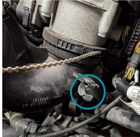
27. Prepare to remove the intake manifold by removing all electrical connections, clips, etc. that will be in the way. This includes the oil pressure sensor plug, rail pressure sensor plug, MAP sensor plug, and rear manifold bracket (2x T25 bolts pictured below, right).
