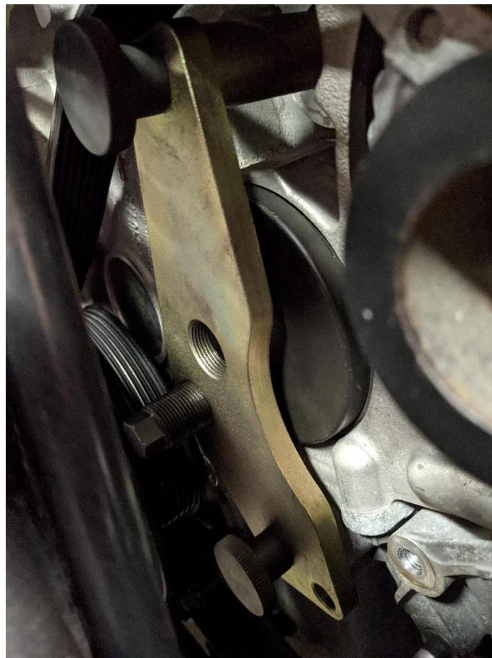
22. Now using a 17mm socket, slowly drive the rounded threaded stud into the plate. As you thread the stud in further, the plate should start angling out. It will need to go in quite far, to reach a sufficient angle to remove the seal.
