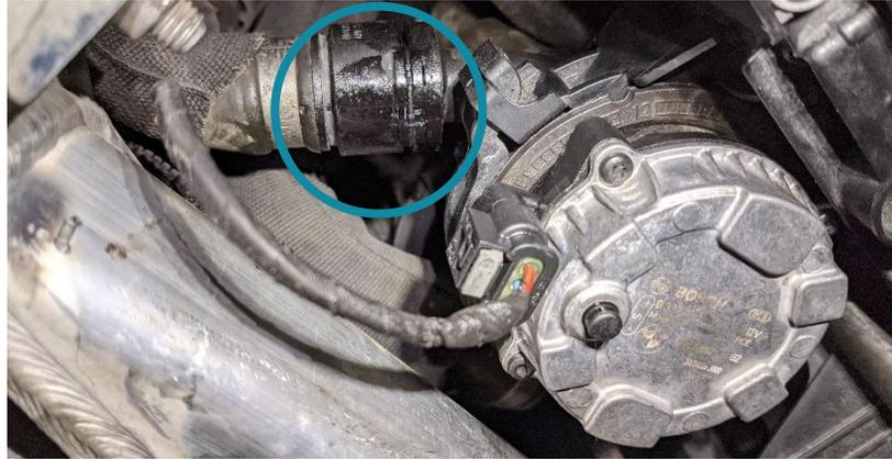
10. Once drained, the intercooler pump can be removed entirely. To do this, remove the single T25 bolt to undo the pump bracket and then lift up. The pump and bracket will come out as one piece. The electrical connection and upper hose connection will also need to be removed:
