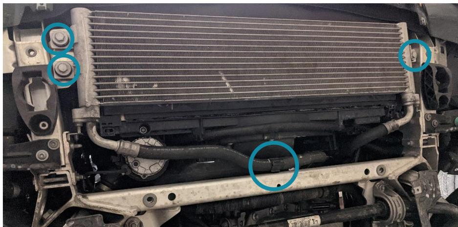
8. Next remove the 2x T25 bolts holding the fan shroud extension and unclip the hose from the fan:
