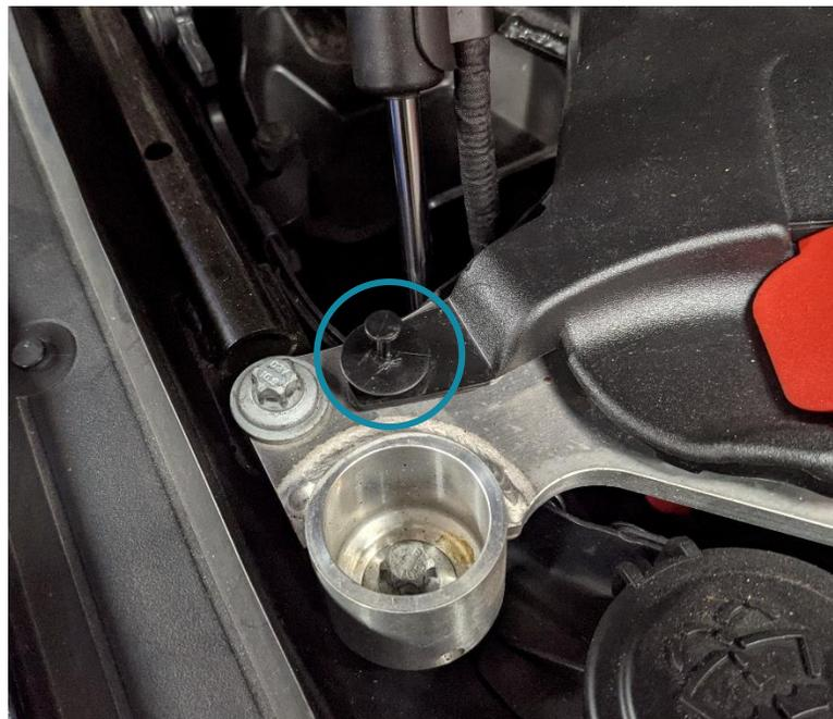
2. Next, remove the cowl weather stripping. First pull the wire out of it's groove and then pull towards the front of the car to remove the weather stripping:
