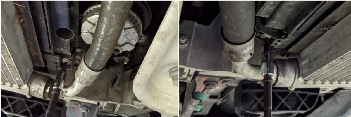
7. Next remove the oil cooler and let it hang freely out of the way. To do this, unclip the hose from the subframe and then remove the 3x 13mm bolts:
