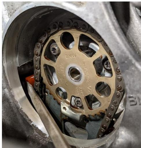
43. Once the gear is back in place, hand-thread the T55 bolt to keep the gear in place. Be sure to clock the vacuum pump assembly outward within its bolt holes. This clocking reference is pictured below and it's important for maximum HPFP to block clearance.
