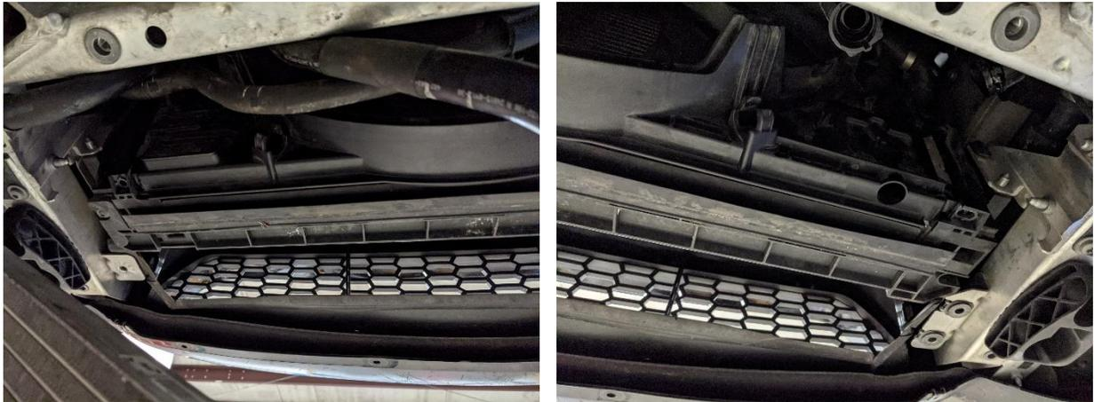
12. Now, moving up top, remove the hose clip from the fan assembly on the left side:
