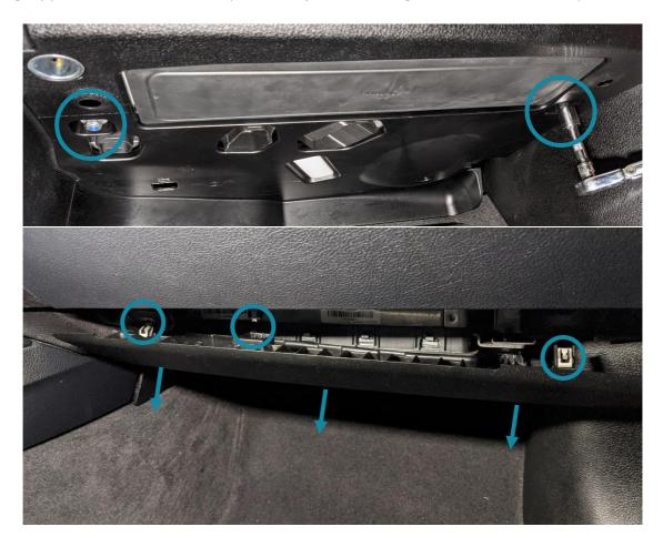
To remove the panel entirely, remove the 12V socket harness and the footwell light harness by simply pulling them out:
