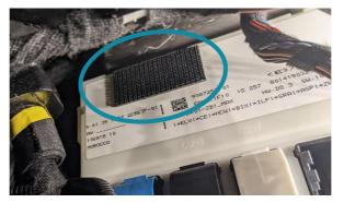
28. Now route the sensor harness (from the engine bay) as shown on the left and connect both the sensor harness and the Dorch signal harness to the Zeitronix ECA.
