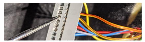
25. You will now have two loose wires on the car's harness (previously removed from the gray connector). Slide these terminals into the small black Dorch supplied connector. Slide the terminals in with their locking tabs facing up towards the hinge on the connector. The connector is marked for position 1 and 2.
