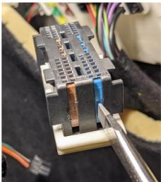
19. One side of this blue connector will be marked with pins 16-27. On this side of the connector, you will swap the terminals out with the supplied Dorch harness (terminal locations and colors are included in the kit and should match the car's original wire colors)
