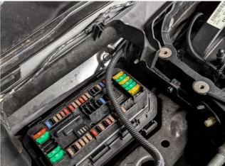
8. Now remove and discard the grommet behind the fuse box (left photo) as this will be the entry point into the cabin. Also, make sure the Dorch supplied grommet has been slid back over the harness in the proper orientation, leaving about 2ft of length from the grommet to the end of the harness (right photo):
