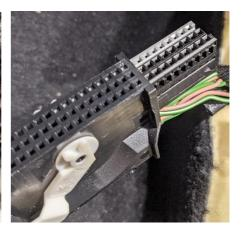
Once the tabs are released, the "Connector B" housing will effortlessly slide off (above right).
