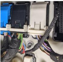
27. Next, stick one side of the supplied adhesive lock-strips to the module (but avoid covering any text/numbers):
