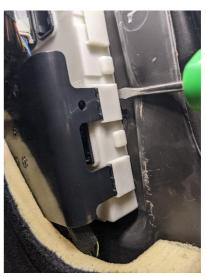
15. (Optional Step) If you'd like to get the cover out of your way, first disconnect the white connector from its mate. Then push the tang down to release the connector from the module cover:
