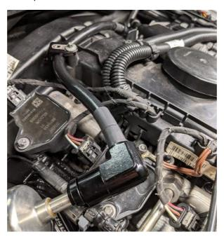
6. The sensor should tuck nicely behind the intake manifold (as pictured below) with plenty of room for the electrical connection. For extra security, 2 zip ties can be used on the sensor itself:
