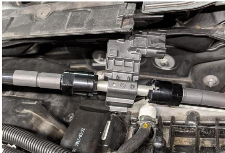
4. Next, connect the elbow fitting to the HPFP by first pushing the fitting onto the HPFP and then threading the collar nut onto the hose.
