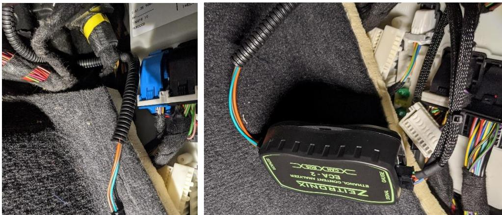
29. Be sure to apply the other side of the adhesive lock-strip to the back of the Zeitronix ECA, and then snap it into place as shown below:
