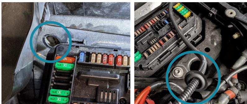
9. Now that the grommet (behind the fuse box) is removed, there will be a layer of foam within the empty hole. Using a long screwdriver or something similar, lightly poke a hole through the foam for your cable entry point.
