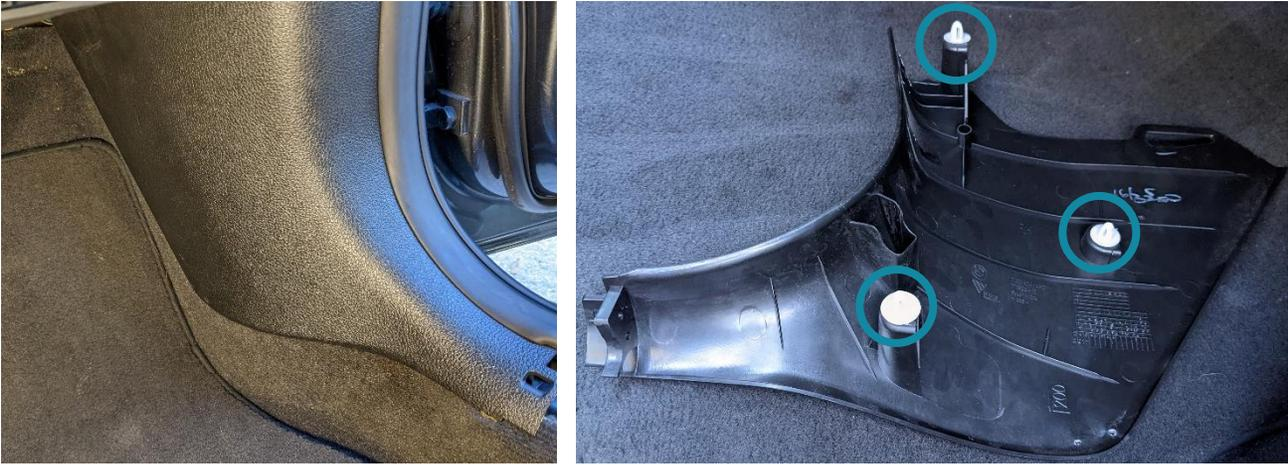
14. Next remove the module cover. There is one T20 Torx, followed by two clips. The clips only have latches on the outer tangs. Push in each outer tang with a screwdriver and pull out to remove the cover:
