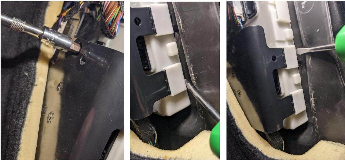
15. (Optional Step) If you'd like to get the cover out of your way, first disconnect the white connector from its mate. Then push the tang down to release the connector from the module cover:
