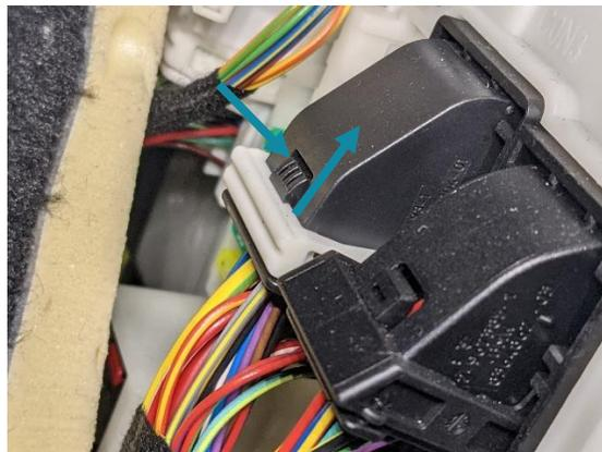
18. Now remove just the blue half of the connector. Take note of the small (blue) tab that locks in the connector. This this can be released by bending out the black housing with your finger (left picture below). Simultaneously lightly push the blue connector out (right picture below). This will slide out effortlessly when the blue tab is free.
