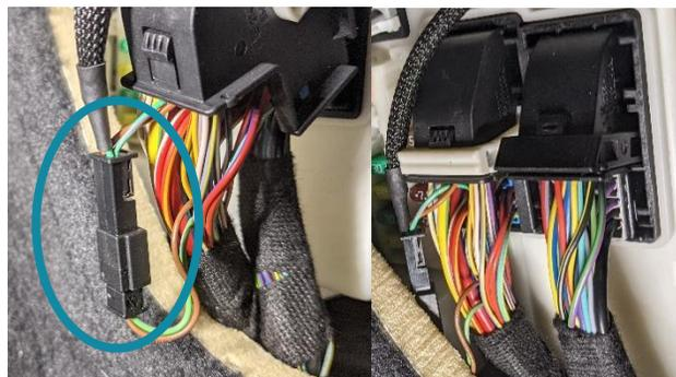
23. The last step is to now repeat the same process for the “Connector B”. Remove “Connector B” from the module and then slide out the black and gray halves. To do this, pull the small tabs outward (left photo below) while simultaneously lightly pushing out with a small screwdriver (center photo below).
