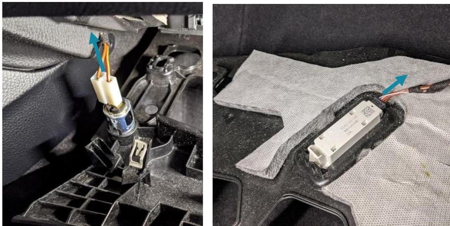
13. Now remove the footwell side panel by pulling directly towards the center of the vehicle at the three clip locations:
