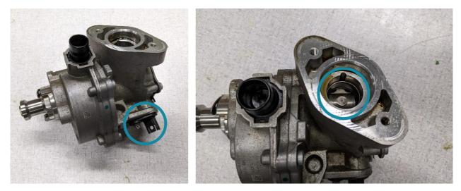
19. Now transfer the cam follower and cam sensor (with O-ring seal) on to the Dorch Engineering supplied vacuum pump assembly. Make sure the follower is oiled when it is dropped into the new assembly.
