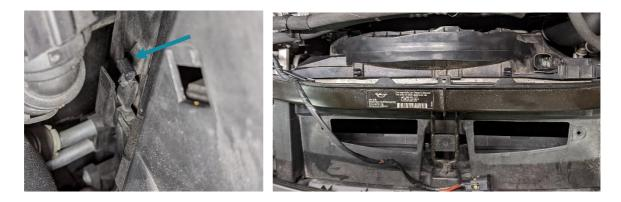
Be sure to lift up slowly with electrical harness and coolant line moved out of the way. Watch for any snags on any other hoses on the lower sections of the fan as it lifts out.
