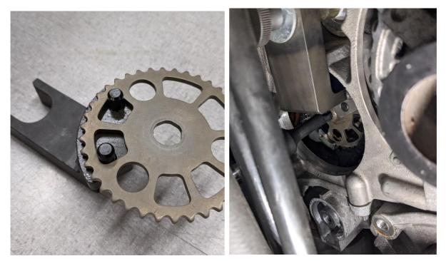
Once the tool is properly locked into the timing gear, use a T55 socket to crack loose the center bolt. Once it is cracked loose, do not remove the bolt. Instead, put it on finger tight and remove the locking tool.
