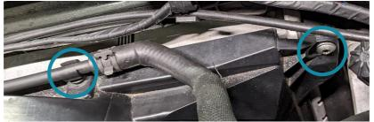
7. The cooling fan assembly is now free to lift upwards and out of the vehicle. When starting to lift the fan, be sure to release the tab on the left side (USA driver's side) of the assembly. Simply push the tab rearward while sliding the fan upward to release.
