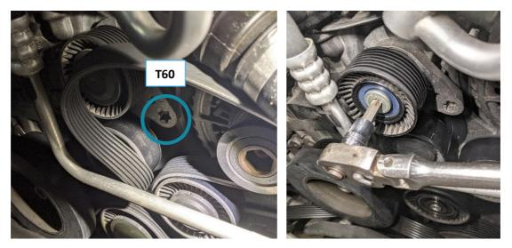
9. Once the tensioner is out of the way, remove the two idler pulleys in the same fashion. First pop off the plastic covers with a pick and then loosen the T50 bolts:
