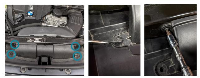
4. Next remove the rear half of the fresh air inlet by releasing the two tabs and pulling away from the airbox
