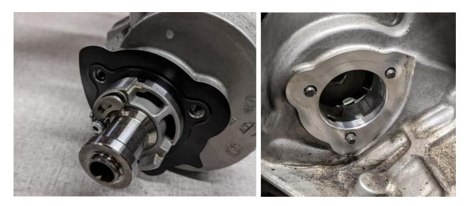
21. The Dorch Engineering vacuum pump assembly can now be installed in the block. Once it is seated in place, the timing gear needs to be placed back on the front of the shaft (reverse process of Step 16). This will require carefully using a screwdriver (again) to hold back the timing chain tensioner while the lining up the gear onto the front of the shaft.
