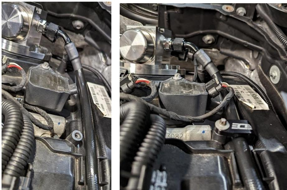
19. **READ THIS STEP THOROUGHLY.** Now install the supplied high pressure line. This line needs to be installed into the rear-most fuel rail port first, then rocked over into the fuel pump port, and lastly pulled down and back into the front-most fuel rail port. It will be a tight fit and the line **MUST BE AS STRAIGHT AS POSSIBLE.**
