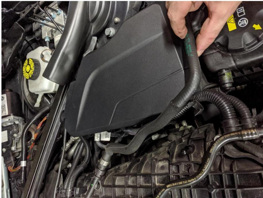
4. Remove the left side strut tower cover clip pictured below (removed) by first pulling up the center and then removing the whole clip. This will give you access to the strut bar bolt.
