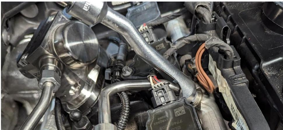
**NOTE:** We don't expect everyone to have specialty sockets for proper torque spec. In this case, simply "snug" the nuts with a 17mm wrench. 31nm is NOT a lot of torque so be sure to not over tighten and damage the line.
