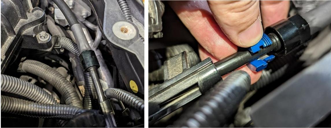
Once the collar is fully threaded on, use a wrench to tighten them. You may need to hold the hose in place by using an additional wrench on the hex portion of the hose fitting.
