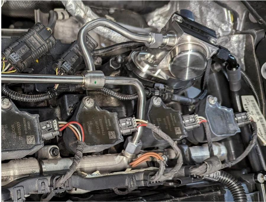
22. At this point, double-check all of your fuel connections, fastener torques, etc. and then reconnect the battery's ground terminal.
