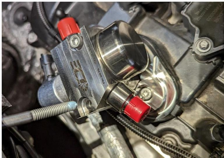
17. Next, install the Dorch low pressure hose. To do this, first push the female hose fitting onto the car's low pressure feed line (left). Then thread the blue collar nut into the hose fitting (right). **Be careful not to drop the collar nut.**
