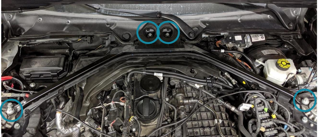
7. Next remove the seven 10mm bolts holding on the upper firewall plastic shroud. There are four bolts on the left side and three on the right:
