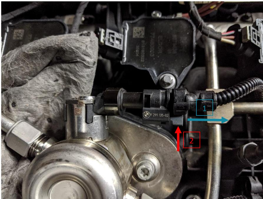
13. The low pressure line can now be removed. Be sure to place a rag under the quick-connect fitting before removal. This fitting requires removal of the gray clip first, and then push the black plastic collar in, while simultaneously pulling the line off.
