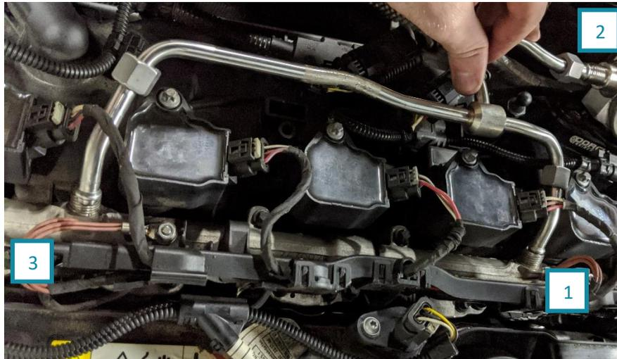
20. Lightly apply oil to the threads of the HPFP to prevent galling. If the nuts thread on effortlessly and bottom out with all the fittings well aligned, the three nuts can now be torqued.
