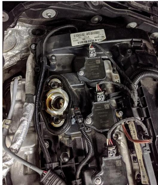
15. Now install the Dorch Engineering pump flange using the supplied Torx T30 bolts and the flange alignment tool. Press the alignment tool into the center of the flange and tighten the bolts.
