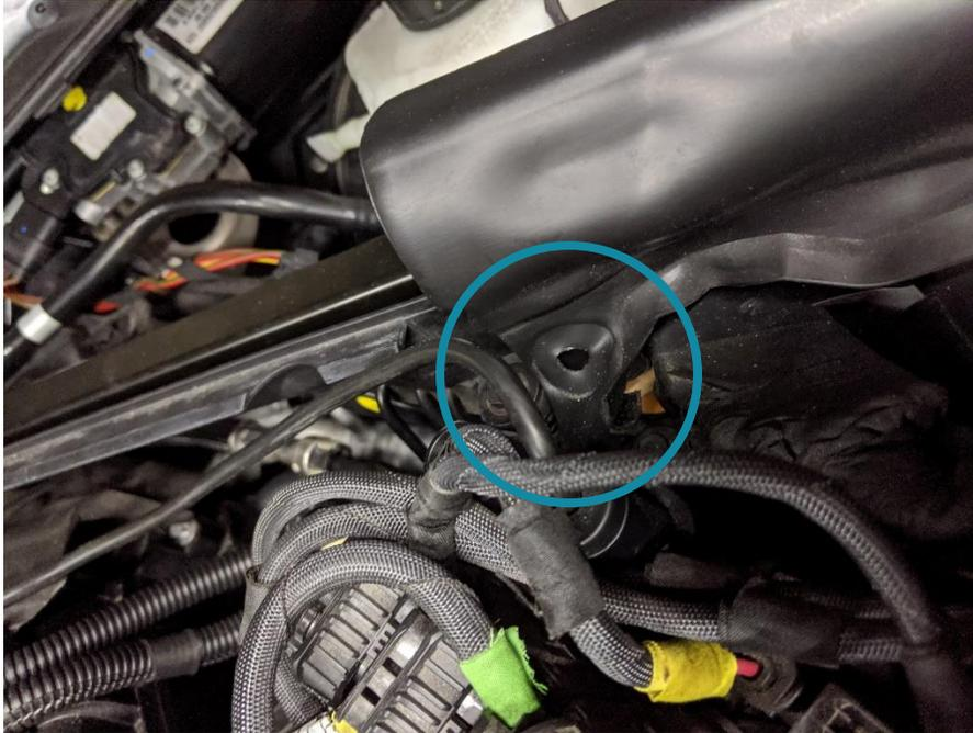
5. To gain access to the strut bar bolts under the cowl, remove the two black circular covers pictured below. These can be removed by reaching underneath and pushing out from the center. Place a hand over top of them as they are pushed out so they don't fly out and get lost.
