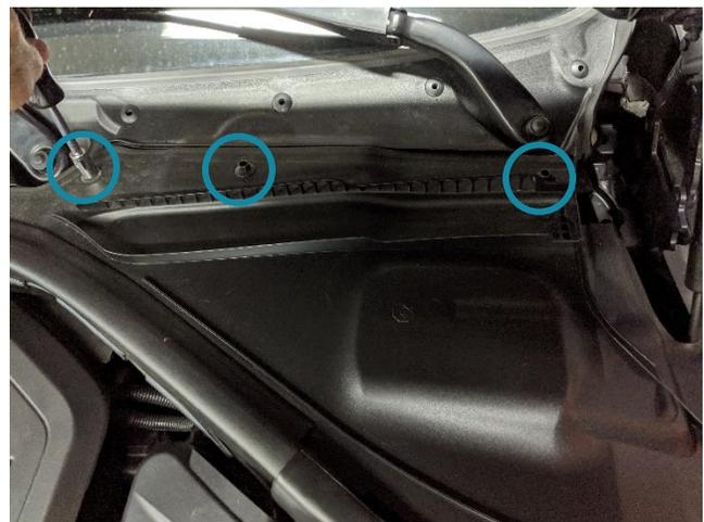
2. Next, remove the cowl weather stripping. First pull the wire out of it's groove and then pull towards the front of the car to remove the weather stripping:
