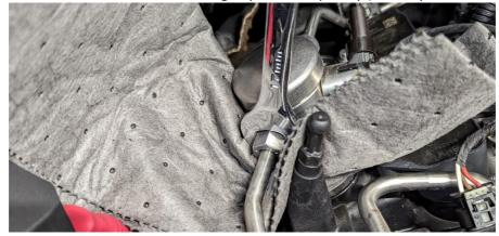
8. Once the high pressure line is drained, it can be removed and you can now move your rag to the low pressure port of the HPFP and crack the 17mm nut loose to ensure the low pressure is drained as well:
