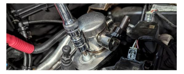
12. Install the Dorch Engineering pump flange using the supplied Torx T30 bolts and the flange alignment tool. Press the alignment tool into the center of the flange and tighten the bolts.
