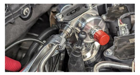
16. Install the Dorch electrical harness adapter as pictured below. Once clicked into place, be sure to push down the gray locking tab on the engine harness (the reverse of step 4).
