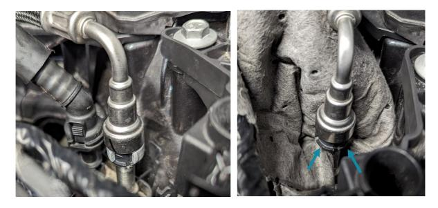
With the gray clip removed, simply push the black release collar into the fitting (upwards) while pulling up on the hose for removal. We recommend another rag here to catch any fuel spillage.
