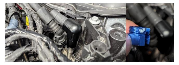
**CAUTION: USE TWO HANDS WHEN THREADING THE BLUE COLLAR NUT.** These can easily be dropped in the engine bay without using caution.
