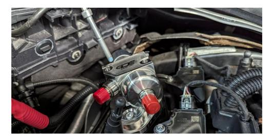
14. **READ THIS STEP THOROUGHLY.** Now install the supplied high pressure line. This line needs to be installed into the rear-most fuel rail port first, then rocked over into the fuel pump port, and lastly pulled down and back into the front-most fuel rail port. It will be a tight fit and the line **MUST BE AS STRAIGHT AS POSSIBLE**.
