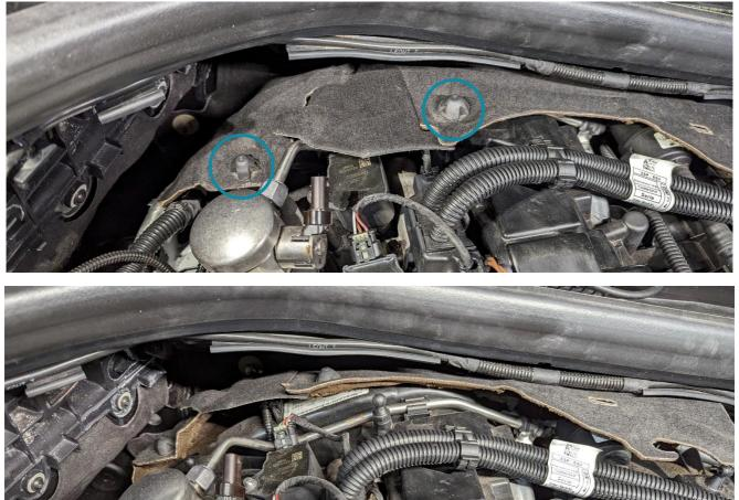
6. Next, using an E6 socket, remove the fastener which is securing the low pressure line to the valve cover:
