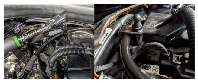
19. With the hose nicely tucked into the OEM groove location, you can now tighten the AN inlet fitting on the HPFP.
