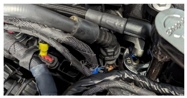
To tighten the collar nut, use a 19mm crow's foot while holding the fitting straight. This just needs to be "snug".
