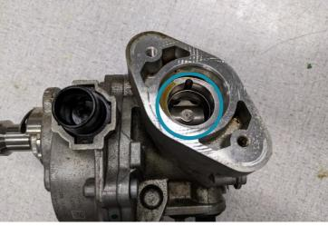
19. Now transfer the cam follower and cam sensor (with O-ring seal) on to the Dorch Engineering supplied vacuum pump assembly. Make sure the follower is oiled when it is dropped into the new assembly.
