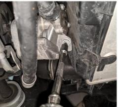
3. Next remove the front half of the fresh air inlet via 2x push pin clips and 2x T25 fasterners:
