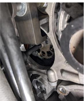
Once the tool is properly locked into the timing gear, use a T55 socket to crack loose the center bolt. Once it is cracked loose, do not remove the bolt. Instead, put it on finger tight and remove the locking tool.
