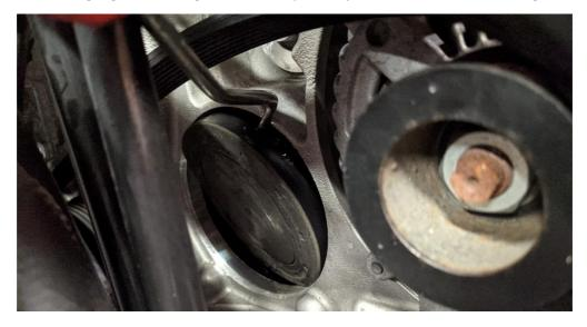
The above sealing cap was finished off with hand tools. By leveraging the bottom in further with the hook, the top edge of the seal became exposed. Once exposed, a long flathead screwdriver and hammer were used to tap downwards on the exposed edge of the seal. This allowed enough rotation to then get the hook in the top (pictured above). Once the top is out, the seal pulls right out.
