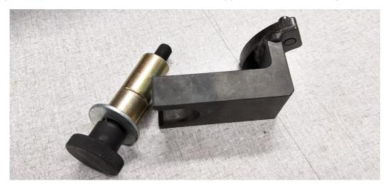
The timing gear can be locked in various positions, but the position pictured below is the most secure. You may need to rotate the engine to get in the proper location to lock the timing gear. To do this, rotate the engine clockwise using a 22mm socket on the crank pulley.
