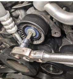
9. Once the tensioner is out of the way, remove the two idler pulleys in the same fashion. First pop off the plastic covers with a pick and then loosen the T50 bolts:
