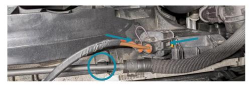
6. Remove the T25 fastener from the upper corner of the fan assembly and release the second clip for the coolant line:
