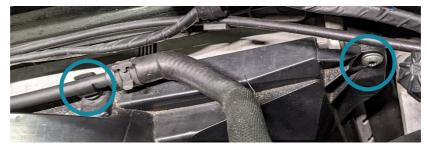
7. The cooling fan assembly is now free to lift upwards and out of the vehicle. When starting to lift the fan, be sure to release the tab on the left side (USA driver's side) of the assembly. Simply push the tab rearward while sliding the fan upward to release.
