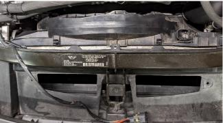
Be sure to lift up slowly with electrical harness and coolant line moved out of the way. Watch for any snags on any other hoses on the lower sections of the fan as it lifts out.
