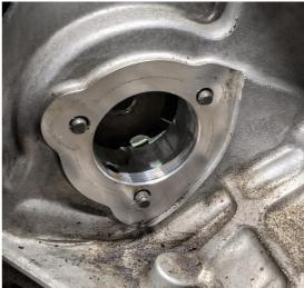
21. The Dorch Engineering vacuum pump assembly can now be installed in the block. Once it is seated in place, the timing gear needs to be placed back on the front of the shaft (reverse process of Step 16). This will require carefully using a screwdriver (again) to hold back the timing chain tensioner while the lining up the gear onto the front of the shaft.
