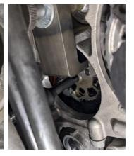
23. Now, reinstall the timing gear lock tool and tighten the center T55 bolt to the final torque.
